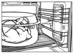
When roasting poultry, the best place to insert the probe is in the thickest part of the meat between the thigh and body.
